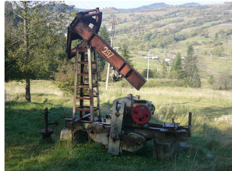
An abandoned oil pump
